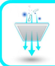
Vertical Laminar Flow system with 30% air recirculation and 70% exhaust system allows operation in sterile and particle free conditions. Thanks to the continuous flushing of the working area by means of a unidirectional vertical HEPA filtered air flow.
